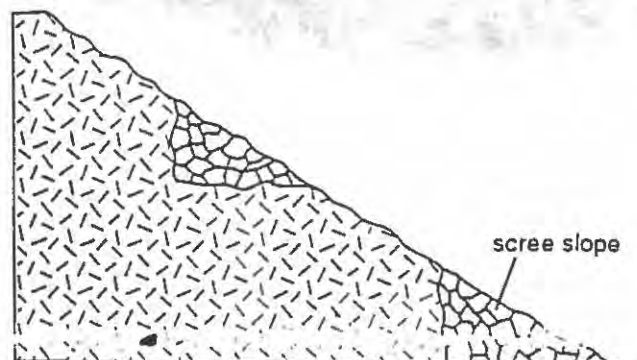
Figure 3. Blasting (top) can reduce or remove benches and create scree slopes (bottom) that can be further stabilized by plantings.
