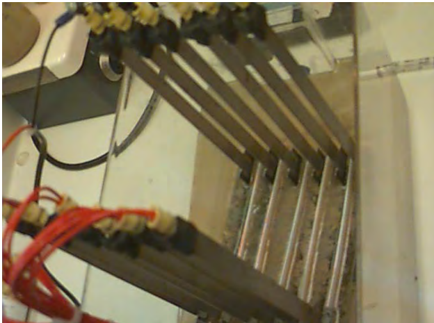
Lab Test Unit showing some floc forming on the surface
