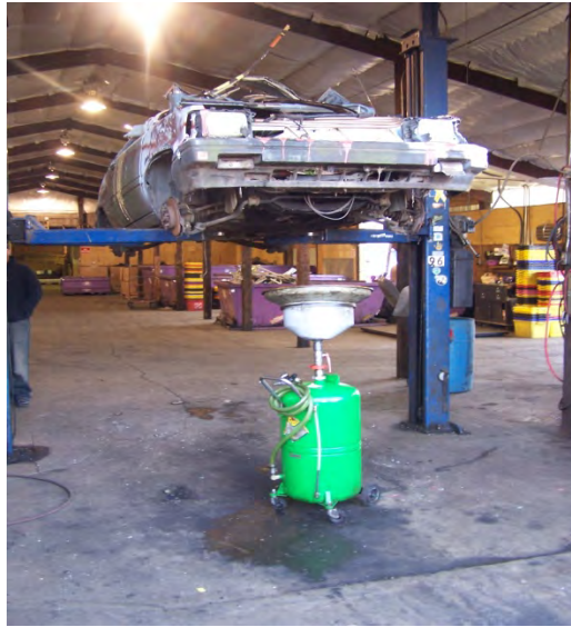
Fluid Gravity Drain System
