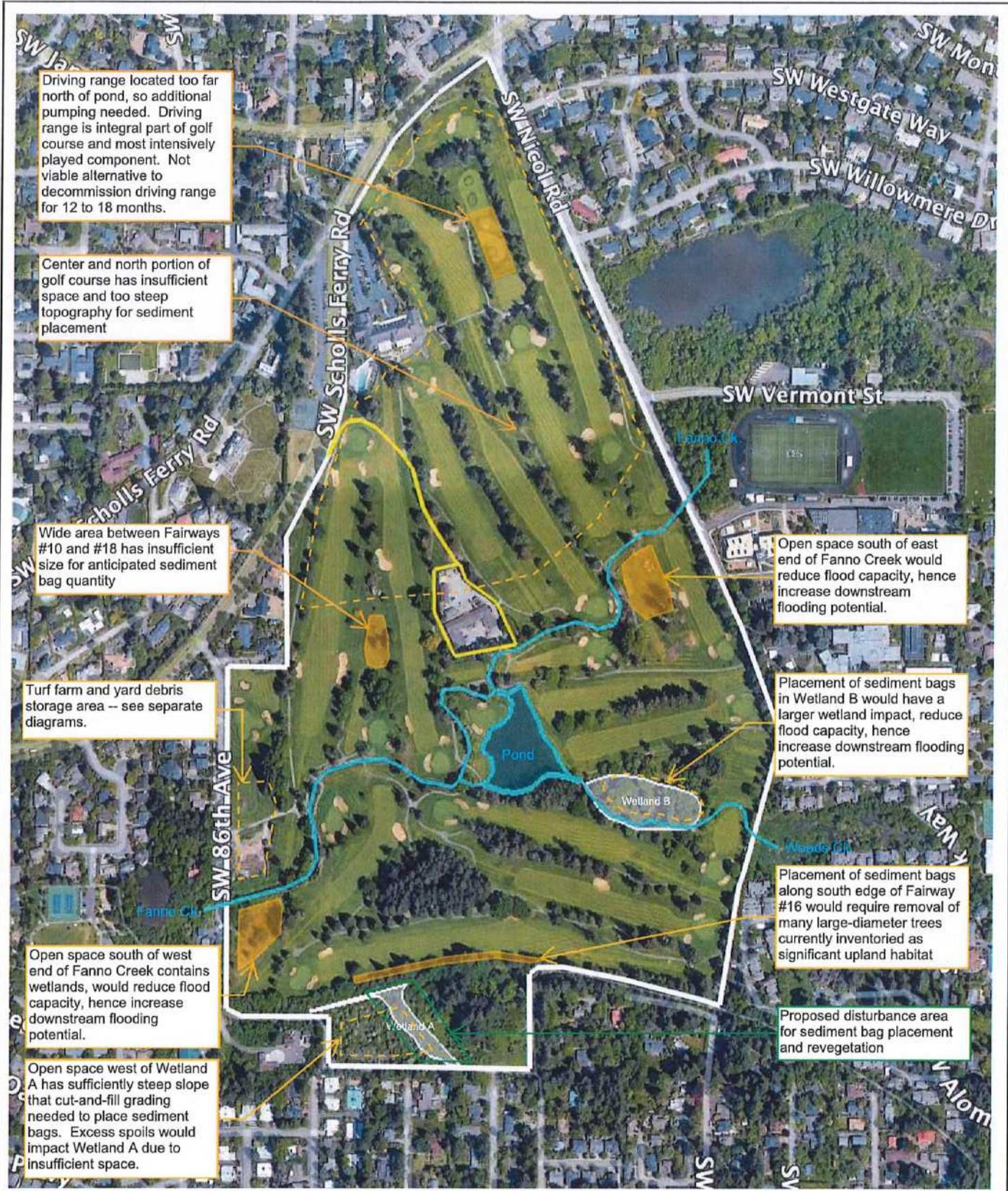
Driving range located too far north of pond, so additional pumping needed. Driving range is integral part of golf course and most intensively played component. Not viable alternative to decommission driving range for 12 to 18 months.
